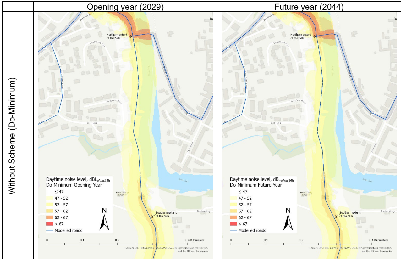
Figure B-1: Predicted absolute noise levels along The Sills for the Do-Minimum Opening Year (top left), Do-Minimum Future Year (top right), Do-Something Opening Year (bottom left) and Do-Something Future Year (bottom right)
